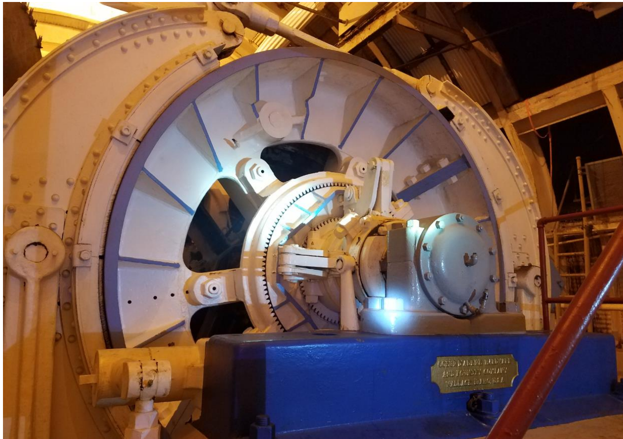
Figure 18-9 #2 Double Drum Coeur d'Alene Hoist
