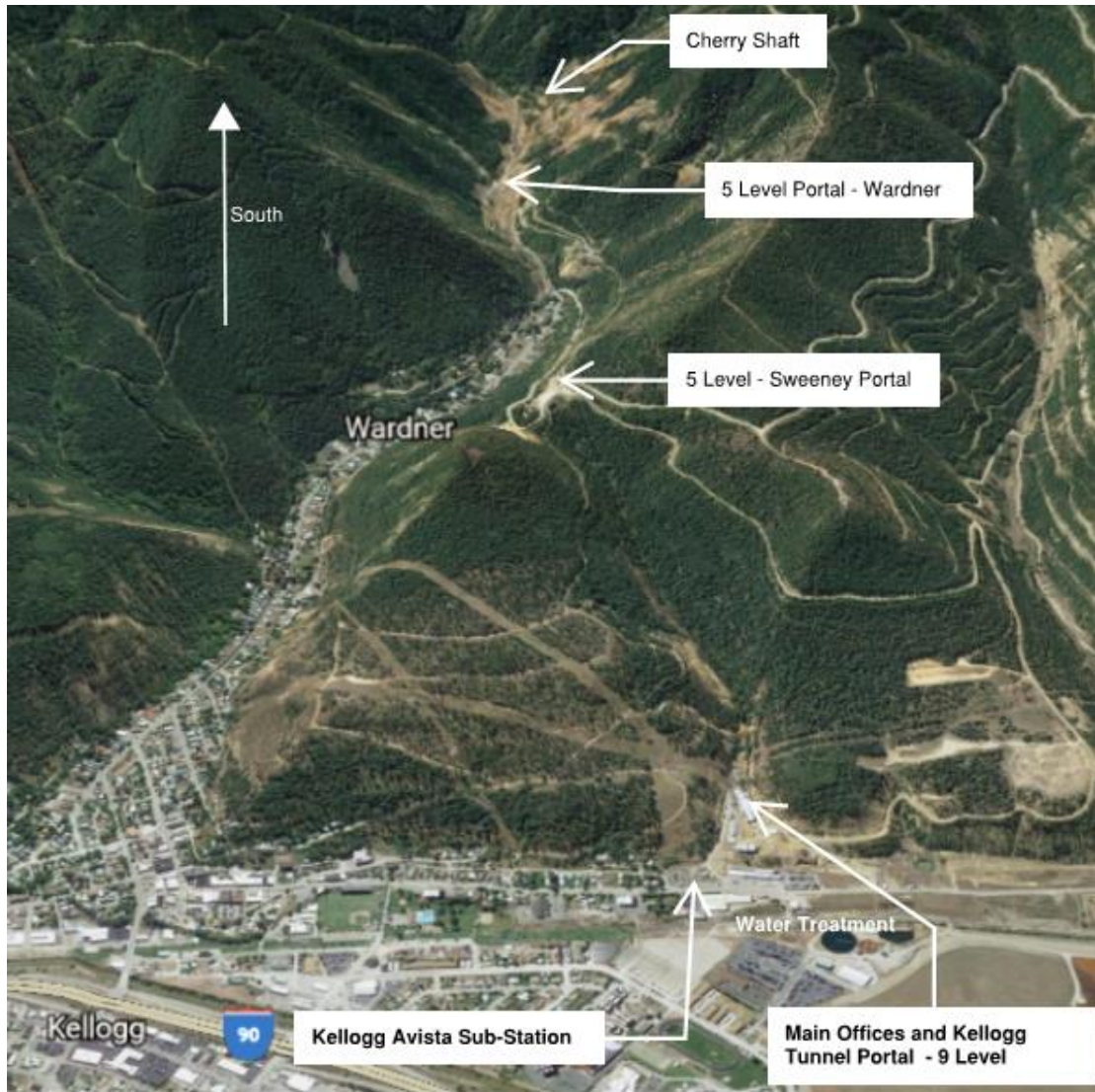
Figure 18-2 Bunker Hill Site Layout
