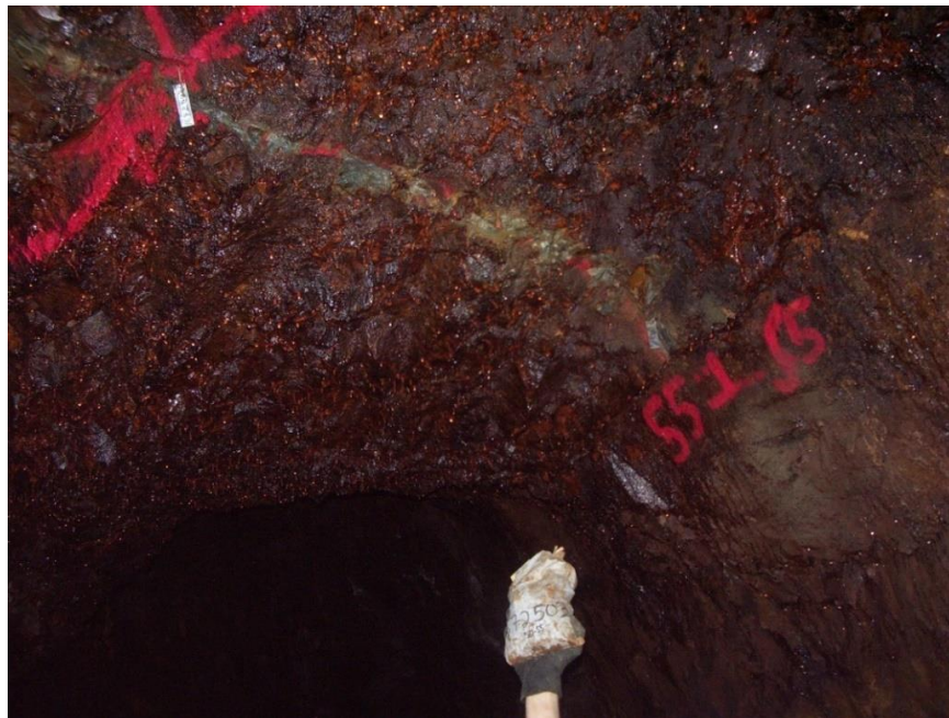
Figure 12-2 Back Sample collected from the 082-25-80 sublevel
