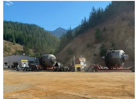
Photo 6: Ball mills arriving by lowboy trailer at Bunker Hill yard
