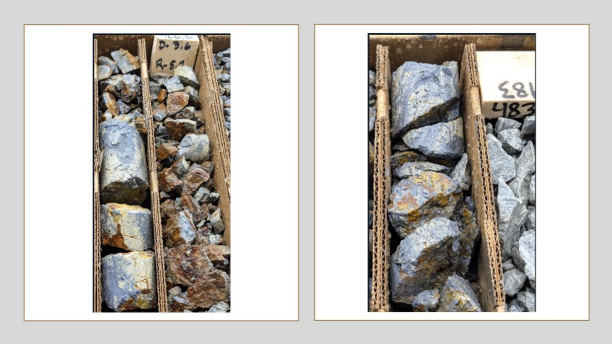
Figure 1: Galena-siderite veins with lead-silver mineralization from BHE26-02. Left photo is 477.3-481.6': 4.3 ft at 8.84 oz/ton (303.09 g/t) Ag, 23.2% Pb, 0.73% Zn (499.7 g/t AgEq). Right photo is 464.5-465.1': 0.6 ft at 5.21 oz/ton (143.64 g/t) Ag, 4.61% Pb, 0.6% Zn (188 g/t AgEq)
