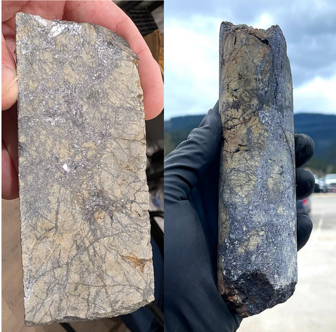
Figure 1: Galena-siderite vein with lead-silver mineralization from 202.8-205.1-foot interval (11.1 oz/ton Ag and 28.4% lead)
