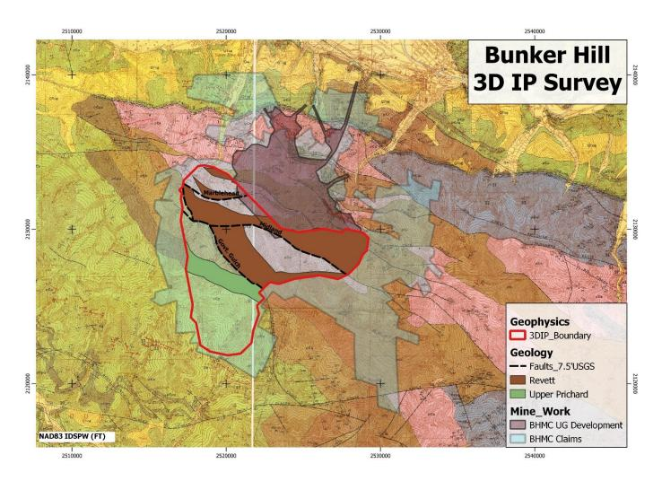
**Image 2:** 7.5' USGS geologic maps for the Smelterville and Kellogg quadrangles with highlighted lithology and major faults over the 3DIP survey boundary.
