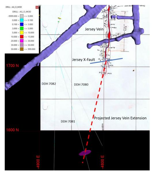
**Image 1:** Geologic map of the 8<sup>th</sup> floor of the 09-Level Jersey Stope showing the cross-cutting fault truncating historic stoping. Drill hole 7081 is shown with vein intercept indicating the extension of the Jersey vein south of the x-fault.
