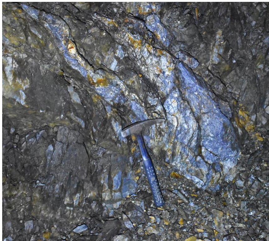
Figure 5: ~18" thick argenteriferous galena-quartz-siderite lens in >30-foot-thick Cate-8 Vein
